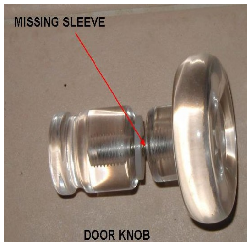
insulating sleeve around openings; missing or out of position.
