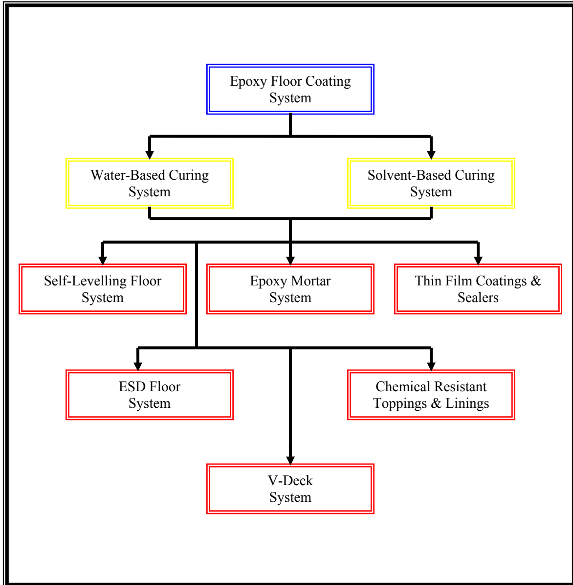
Figure 7 - Types of epoxy floor coating system
