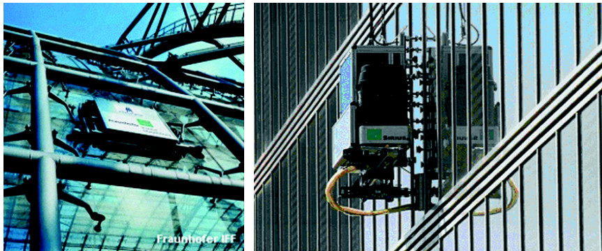
Figures 5.25. Cleaning robots on glass facades (Courtesy of: Fraunhofer Institute for Factory Operation and Automation IFF).
