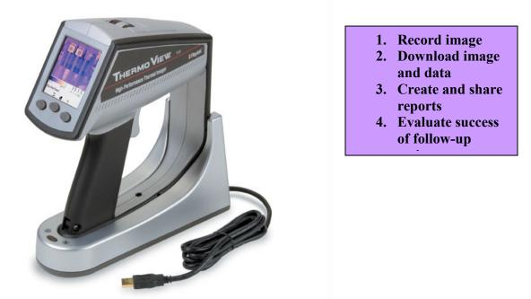
Preventive and predictive maintenance programs can greatly minimize repair and labour costs, reduce inventory of parts, and avoid product variation and production loss. Thermal imaging has emerged as an effective predictive maintenance technology by identifying variations that can lead to equipment failure.
