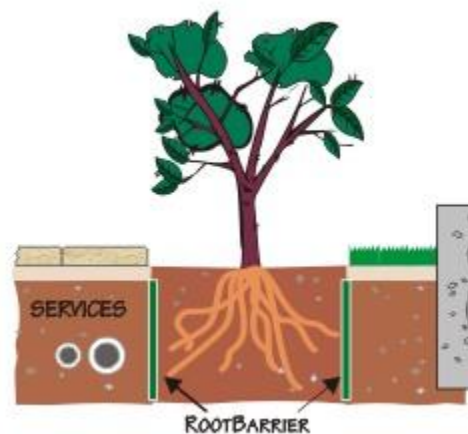
Figure 21: Root Barrier to contain the plant roots
