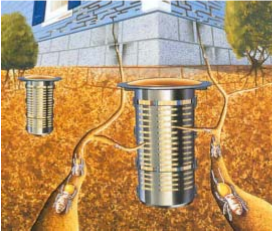
Figure 29: Another method of post treatment control is baits. Baits include Sentricon, FirstLine, and Exterra. Bait stations are spaced anywhere from 12" to 2' apart, depending on the material. Bait stations are environmentally friendly because very little chemical is needed. However, it is sometimes a slow process because termites must find the bait station for this treatment to be effective.
