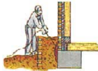
Use rod injection to treat soil along and around the external perimeter area of the building
