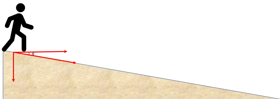
Figure 3 Higher slip resistance required on a slope
